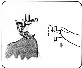
Release lever and commence forward sewing guiding fabric by hand as it is fed. Never pull material.
